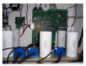
Inverters have capacitors that store energy which is discharged soon after power to the inverters is disconnected.
