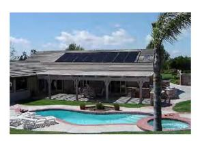
heat collection. Individual panels are lightweight (less than 75 pounds). Multiple panels are connected together. Most systems will use enough panels to roughly equal one-half of the surface area of the swimming pool (a 20' by 30' swimming pool has a surface area of 600 square feet so a typical solar pool heating system would use about 300 square feet of solar panels). Plastic flexible panels can be cut through or easily removed for ventilation operations.
