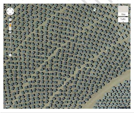
Figure 6: The Ivanpah Solar Electric Generating System as seen via satellite. The mirrored panels are  $5 \times 8$  feet.
