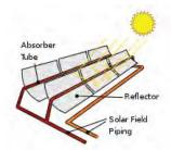
2) Trough systems are composed of parabolic mirrors which focus and reflect the sun to a tube that converts the heat from the sun into electricity. The perceived threat to birds is associated with the presence of water ponds which attract birds and from traumatic impact with the trough structures. An example of this type of solar power plant is Genesis Solar Energy Project.
