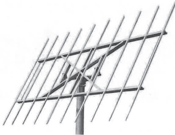
Typical dual axis mounting structure
