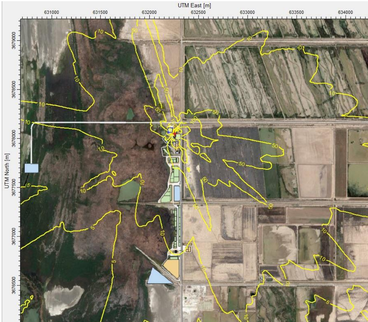
FIGURE A-4 8-HOUR CO CONCENTRATIONS FROM PROJECT STARTUP
