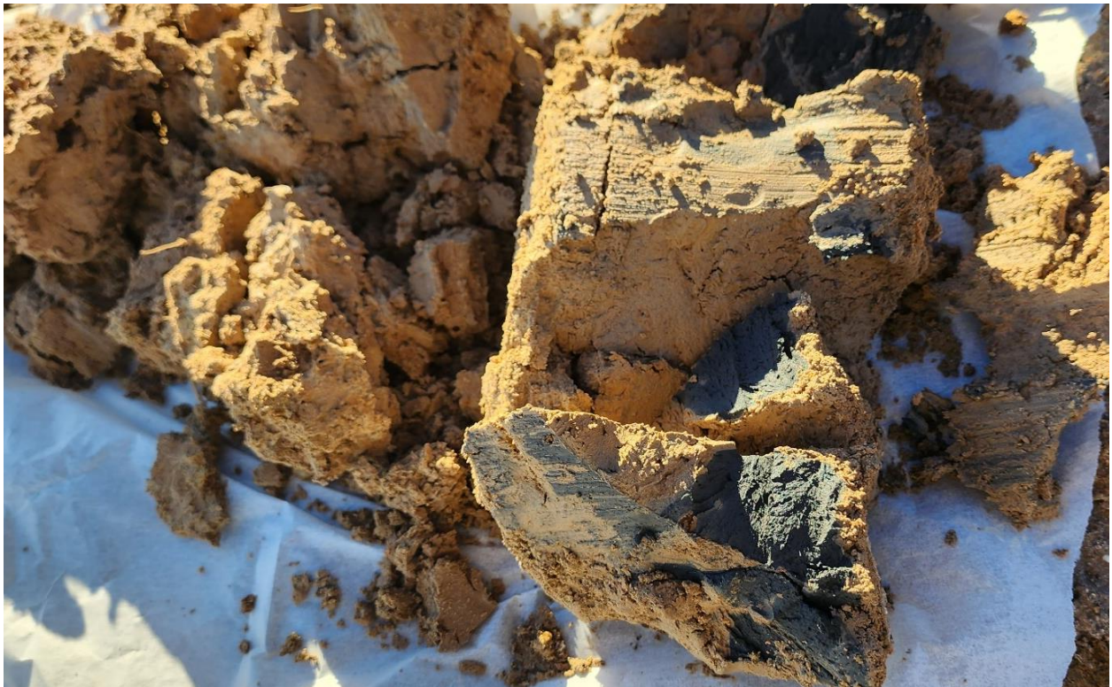
Photo 2: View of clay loam soils with depleted matrix (F3) at W1.
