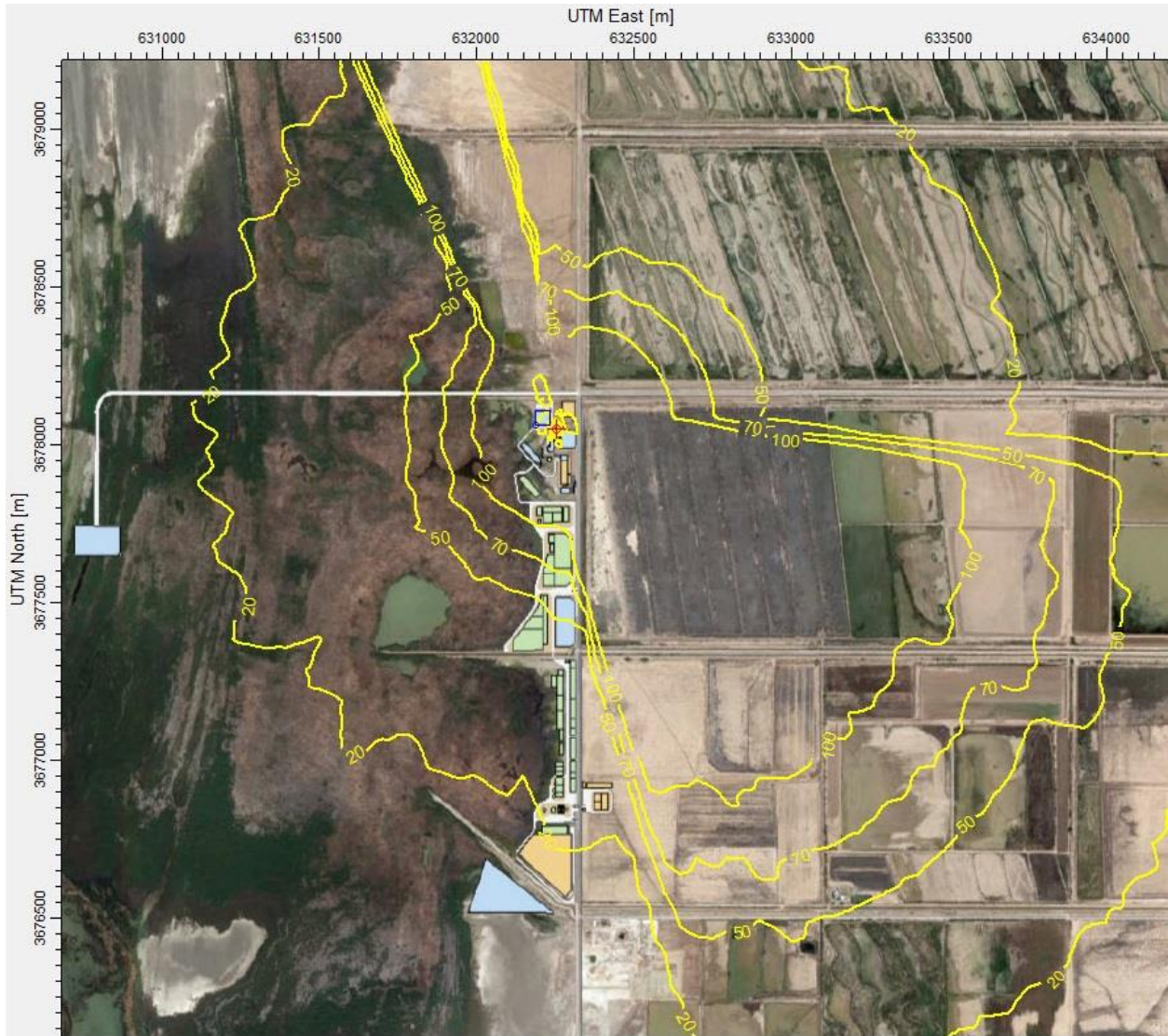
FIGURE A-3 1-HOUR CO CONCENTRATIONS FROM PROJECT STARTUP
