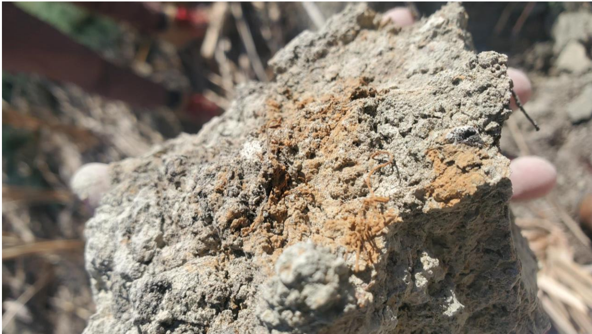
Photo 4: View of redox features in clay loam soils at WPF-2.
