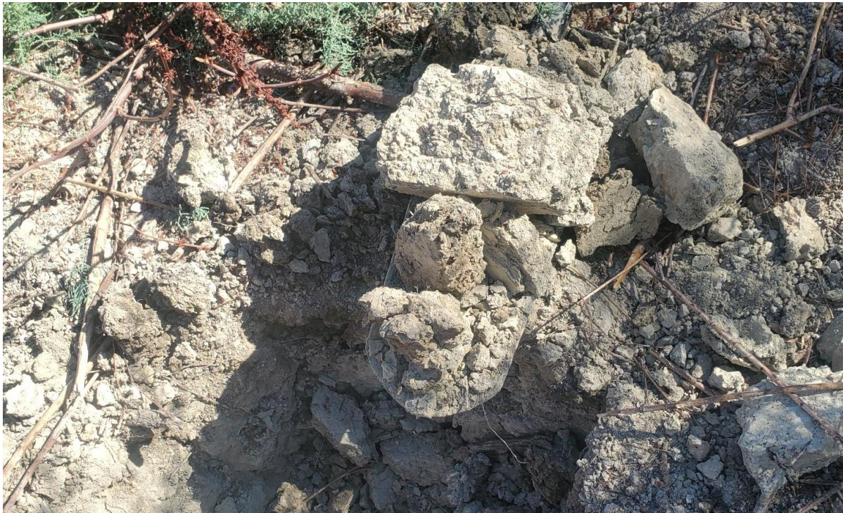
Photo 2: View of silty clay loam soils with redox depression (F8) at WPF-1.
