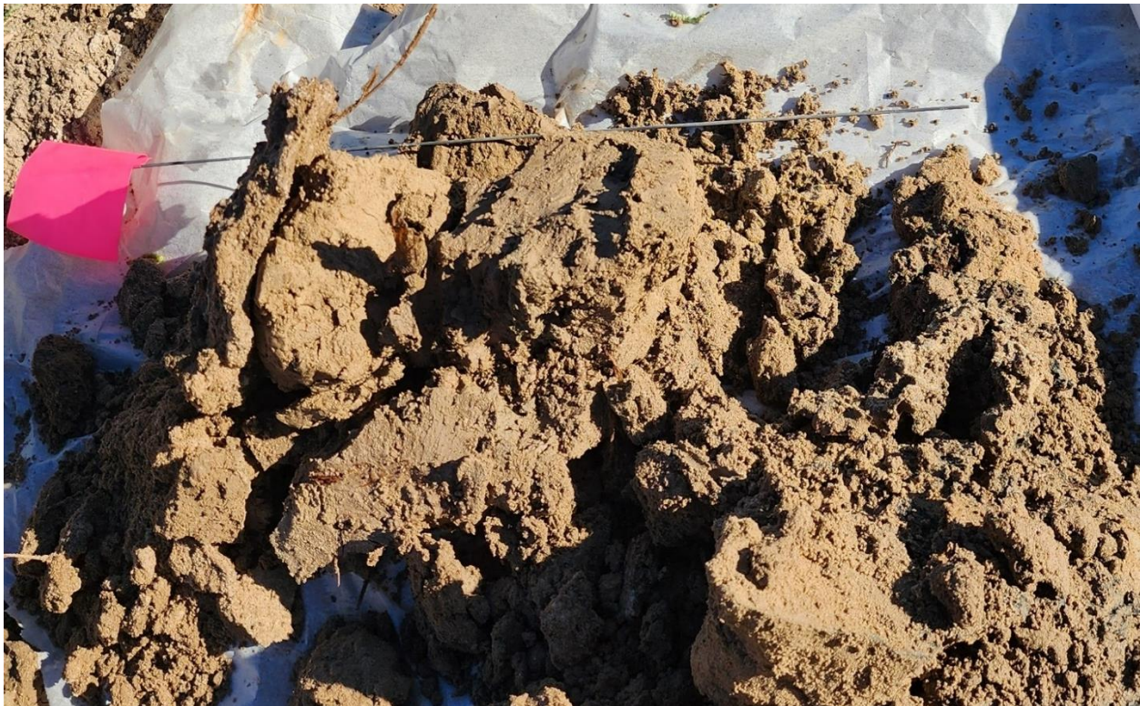
Photo 4: View of sandy clay loam soil cross-section at U1.
