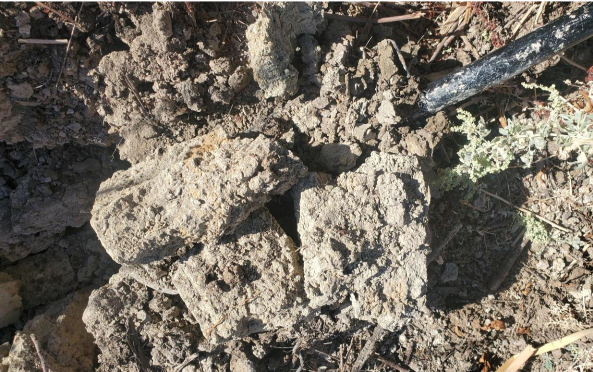
Photo 6: View of hydric clay loam soils with redox features in matrix and pore linings at WPF-3.
