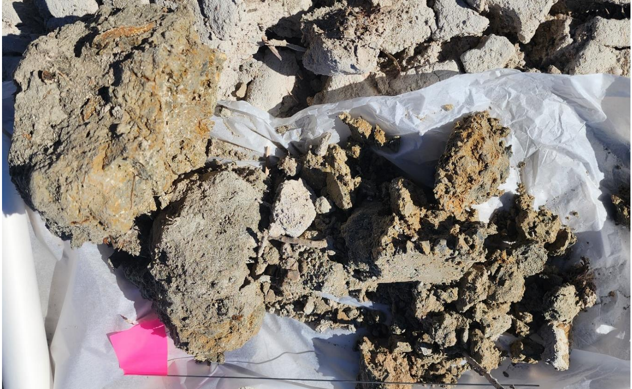
Photo 11: View of redox matrix (F8) at W4.
