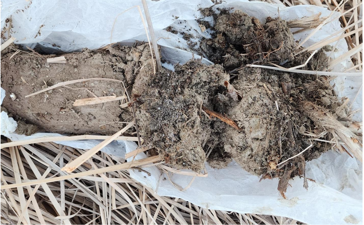
Photo 25: Soil cross section with redox depressions (F8) at W8.
