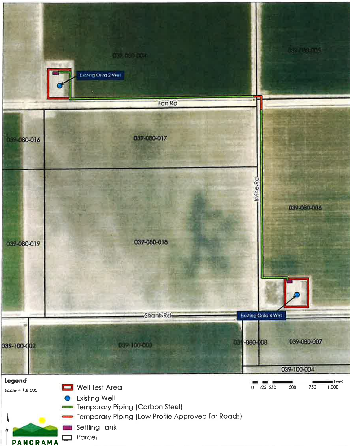
Figure 2 Proposed Temporary Pipeline Alignment
