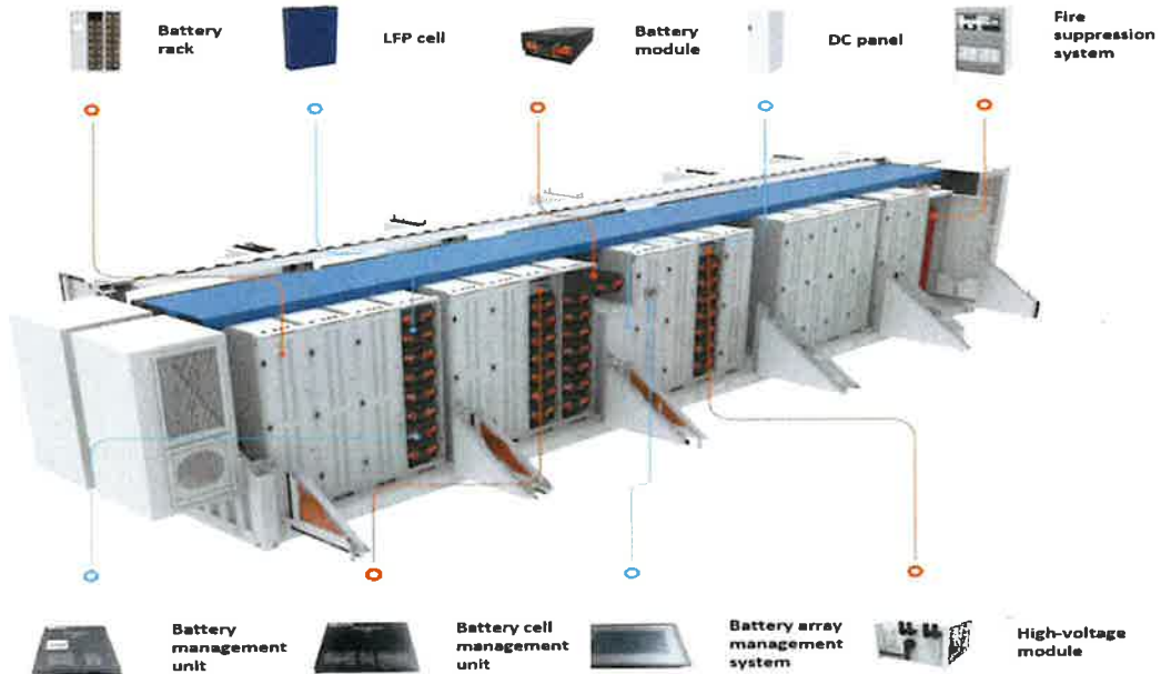
Typical arrangement of a self-contained BESS with battery, inverter & transformer
