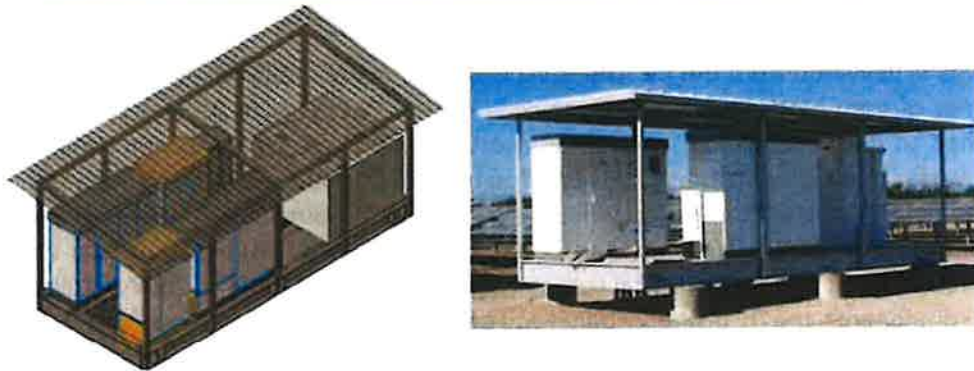
Typical inverter stations
