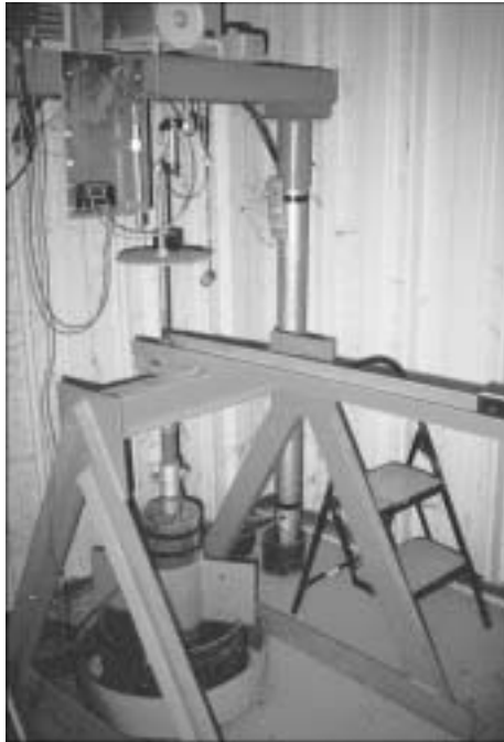
Figure 19 Photograph of extensometer
